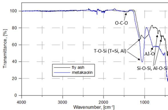
Figure 6. FT-IR spectra of raw materials
