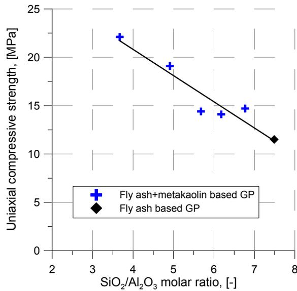
Figure 2. Effect of  $\text{SiO}_2/\text{Al}_2\text{O}_3$  molar ratio
